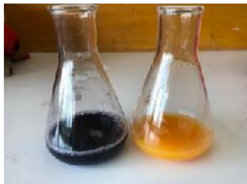
Fig. 2. Titration result of the Vitamin C concentration; (Right side) before of titration (Left side) after of titration
