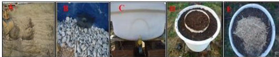
Fig. 3. Soil collection area to fill lysimeters (A), gravel and coarse sand layer (B), drain outlet (C), lysimeter filling with the cylinder in the center (D) and cover with crushed corn husk (E).
