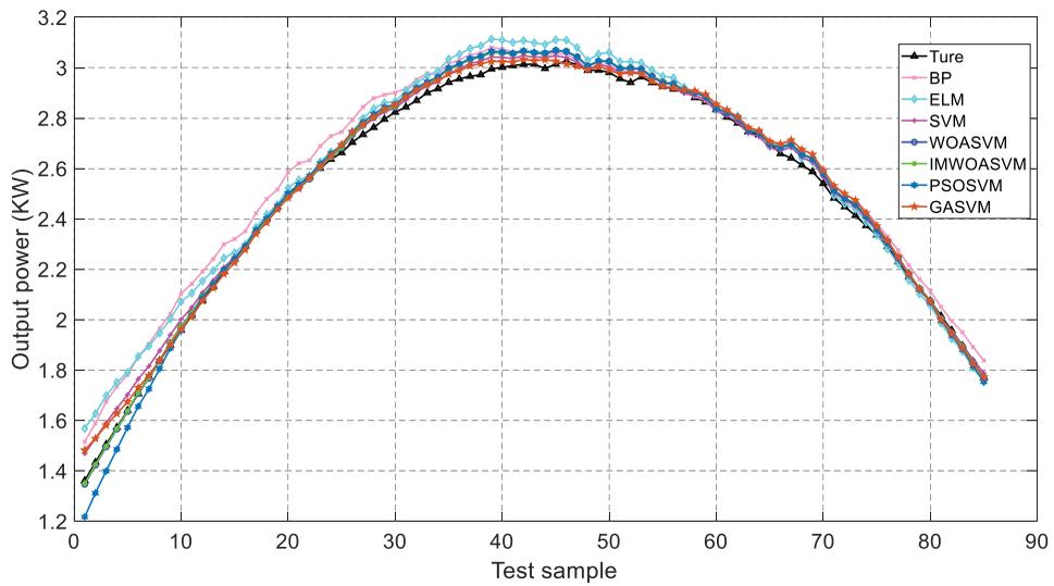
**Figure 5.** PV output power forecast in sunny weather.
