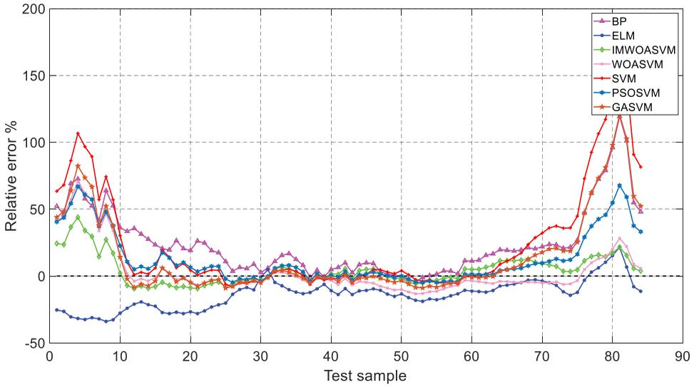
**Figure 8.** Prediction relative error of output power in cloudy weather.
