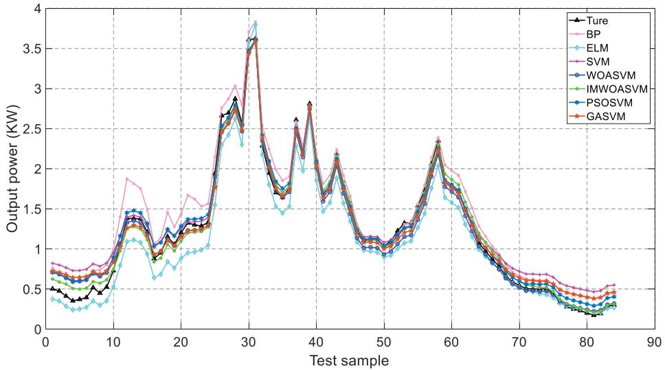
**Figure 7.** Output power forecast in cloudy weather.
