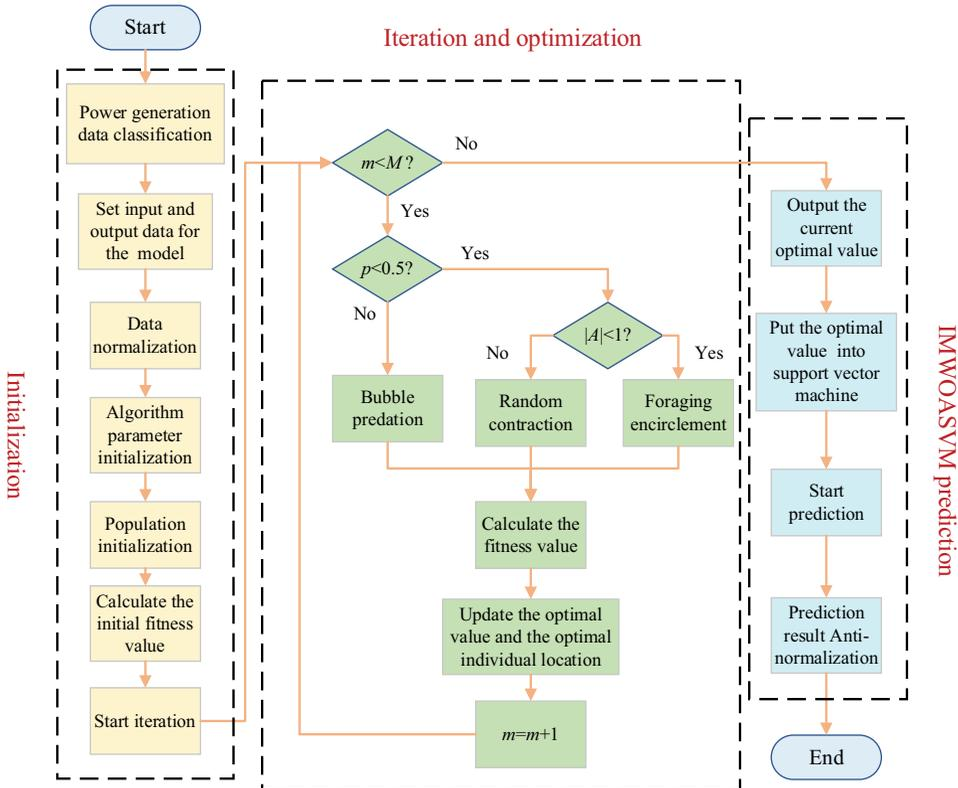
Figure 2. Flow chart of photovoltaic power output predicted by IMWOASVM model.
